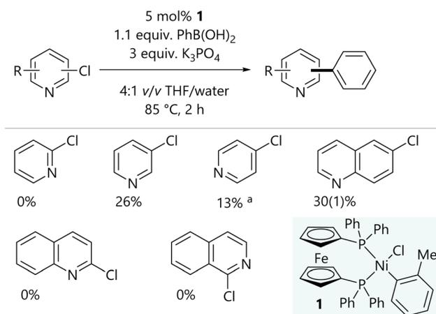
**Scheme 2** Initial attempts at the Suzuki–Miyaura reaction of chloroheteroarenes. Results are quoted as conversion to product as determined by calibrated GC-FID analysis. <sup>a</sup>Substrate was used as the hydrochloride salt, so 4 equiv.  $\text{K}_3\text{PO}_4$  were used.
