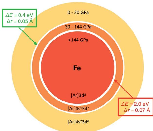
Fig. 3 Example of the relationship between atomic radius and total energy. The size of the Fe atom at different pressures is to scale. White regions correspond to [Ar]4s<sup>2</sup>3d<sup>6</sup> ( $S = 2$ )  $\rightarrow$  [Ar]4s<sup>1</sup>3d<sup>7</sup> ( $S = 2$ ) and [Ar]4s<sup>1</sup>3d<sup>7</sup>  $\rightarrow$  [Ar]3d<sup>8</sup> ( $S = 1$ ) ground state configurational transitions predicted at 30 and 144 GPa, respectively.
