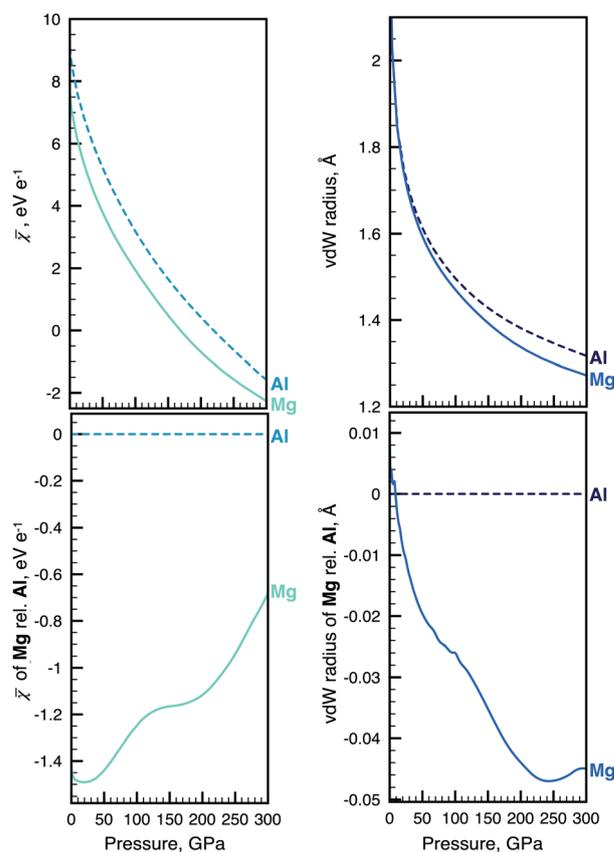
Fig. 1 Example of the sometimes complex relationship between atomic radius and electronegativity. Absolute changes in  $\bar{\chi}$  (top left) and radius (top right) of Mg and Al during non-reactive compression. The same data for Mg is shown relative to Al for  $\bar{\chi}$  and radius at bottom left and right, respectively. The pressure evolution of radii and electronegativity for other atoms can be visualized with the AUP database.<sup>59</sup>
