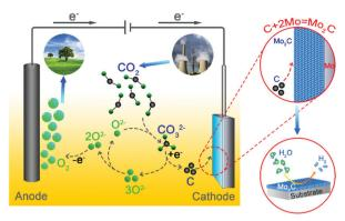
Fig. 1 Schematic illustration on electrochemical fixation of CO<sub>2</sub> in molten salts over a Mo substrate to prepare functional Mo-C films.
