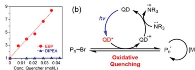
**Fig. 5** (a) Stern–Volmer plot of QD fluorescence ( $\lambda_{\text{ex}} = 460$  nm) effectively quenched by EBP but not by DIPEA. (b) Proposed oxidative quenching mechanism of ATRP catalyzed by CdSe QDs. Reproduced from ref. 61 with permission from the American Chemical Society, copyright 2018.
