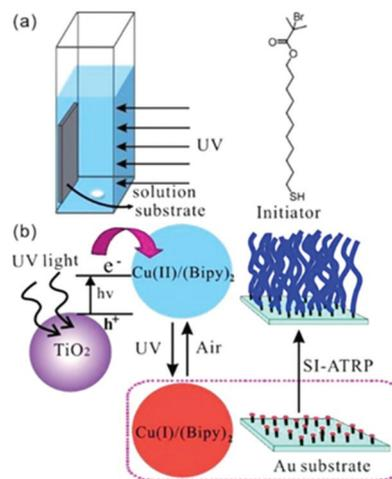
Fig. 3 Scheme of the reaction setup, initiator, photoinitiation mechanism and brush formation via surface-initiated ATRP using  $TiO_2$  NP as the photocatalyst. Reproduced from ref. 71 with permission from the American Chemical Society, copyright 2013.
