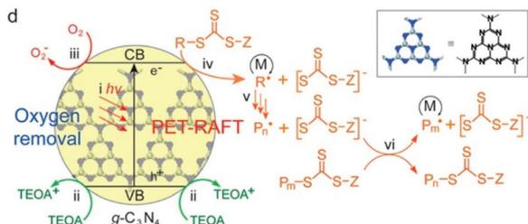
**Fig. 13** Proposed mechanism of PET-RAFT polymerization using g-C<sub>3</sub>N<sub>4</sub> as the photocatalyst in the presence of TEOA. Reproduced from ref. 36 with permission from the American Chemical Society, copyright 2017.
