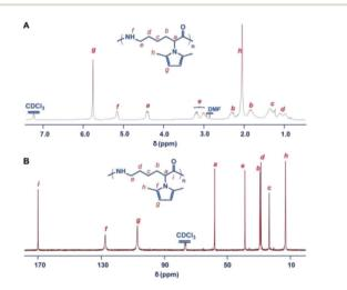
Fig. 3 Structure characterization of the polymer of the 2,5-dimethylpyrrole protected  $\alpha$ -amino- $\varepsilon$ -caprolactam monomer. (A) <sup>1</sup>H NMR spectrum of the polymer. (B) <sup>13</sup>C NMR spectrum of the polymer. The polymer was obtained with sodium (0.5%) in bulk at 260 °C. All spectra were measured in CDCl<sub>3</sub> at room temperature. Reproduced from ref. 25 with permission from the Royal Society of Chemistry, copyright 2015.
