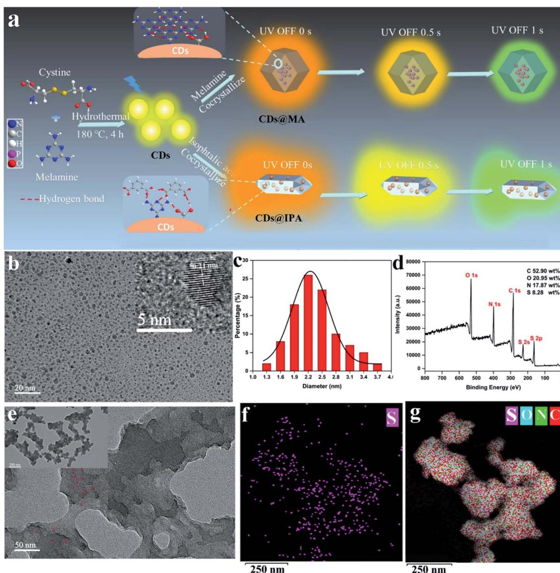
**Fig. 1** (a) Scheme for the synthesis and luminescence properties of CDs@MA and CDs@IPA composites. (b) TEM image of CDs. Inset: HR-TEM lattice fringe image of CDs. (c) Size distribution of CDs. (d) XPS survey spectrum of CDs. (e) TEM images of CDs@MA. The EDX maps of (f) S and (g) C, N, S, O elements in CDs@MA.
