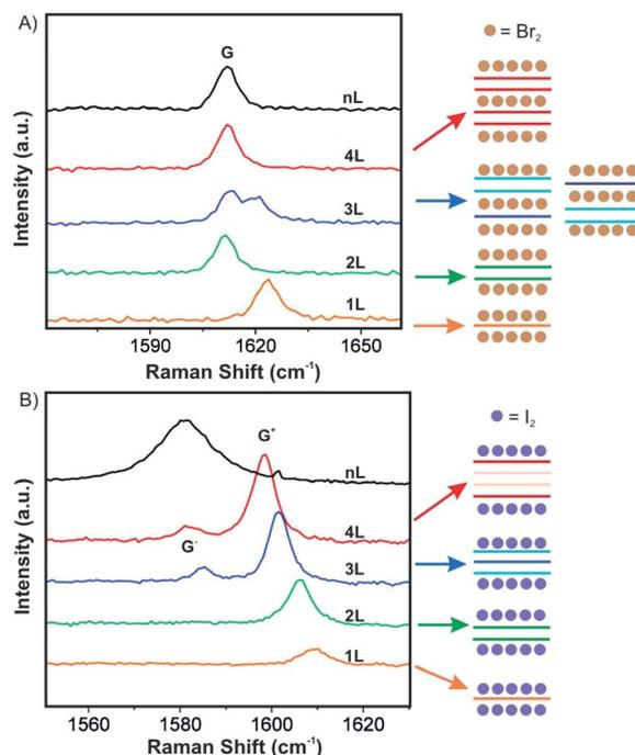
Fig. 8 Raman spectra of few layer graphene materials exposed to (A) Br<sub>2</sub> and (B) I<sub>2</sub> and the derived intercalation models. Adapted from ref. 50 with permission from the American Chemical Society, Copyright 2009.
