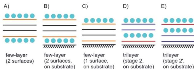
Fig. 3 Concept of few-layer surface functionalization/intercalation. (A) Surface functionalized few-layer material, here the interior 2L differ from the outer layers; (B) as in (A), but with substrate influence leading to Janus-type properties; (C) few-layered material with intercalation only on the top; (D) and (E) illustration of stage 2 and stage 2' intercalation for 3L materials.
