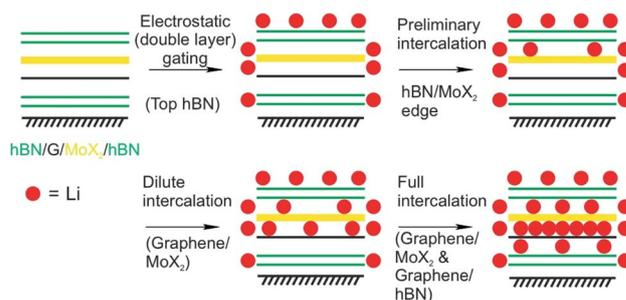
Fig. 24 Proposed four-step Li intercalation mechanism for a hBN (green)/MoX<sub>2</sub> (yellow)/graphene (black)/hBN heterostructure, evidenced by *in situ* HRTEM imaging.<sup>87</sup>
