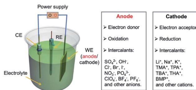
Fig. 12 Configuration of an electrochemical cell for bulk intercalation and typical reactions as well as typical intercalants. Reproduced from ref. 81 with permission from Wiley-VCH Verlag GmbH & Co, Copyright 2020.
