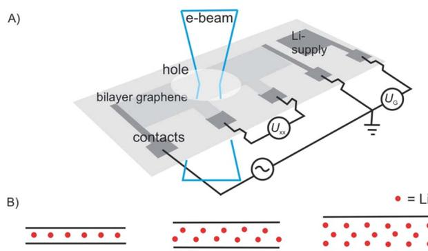
Fig. 1 Illustration of *in situ* transmission electron microscopy of the Li-intercalation process in suspended 2L graphene, triggered in a device. (A) Illustration of the device on a  $\text{Si}_3\text{N}_4$ -covered Si substrate. (B) from left to right: side-views of expected ‘conventional’  $\text{C}_6\text{LiC}_6$  configuration and of the experiment matching structures with 2L Li crystal and 3L Li crystal.<sup>15</sup>
