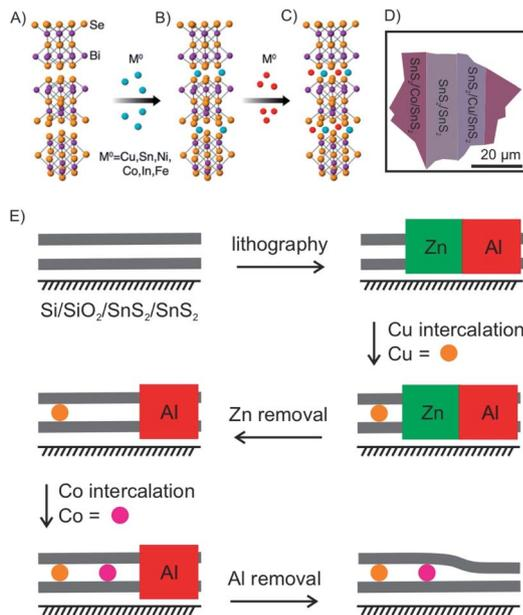
**Fig. 11** Intercalation of (A and B) single and multiple (C) zero-valent metal atoms into  $\text{Bi}_2\text{Se}_3$ . Adapted from ref. 66 with permission from the American Chemical Society, Copyright 2015. (D) Schematic illustration of seamlessly integrated n-type  $\text{SnS}_2$ , p-type  $\text{Cu-SnS}_2$  and metallic  $\text{Co-SnS}_2$  within a single nanosheet. (E) Schematics of the spatially controlled intercalation process for 2L  $\text{SnS}_2$ .<sup>67</sup>
