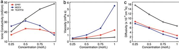
Fig. 3 The ionic conductivity (a), viscosity (b), and diffusivity (c) of EPRT-TFSI, MEEV-(TFSI)<sub>2</sub>, and TEATFSI at 0.25, 0.50, 0.75, and 1.00 M in ACN. The uncertainties associated with measurements are reported in the Table S1 (ESI†), as the uncertainty bars are smaller than the symbol size on the graphs.
