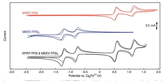
Fig. 4 Cyclic voltammograms of EPRT-TFSI (red, top traces), MEEV-(TFSI)<sub>2</sub> (blue, middle traces), and an equimolar combination of both EPRT-TFSI and MEEV-(TFSI)<sub>2</sub> (black, lower traces) at 10 mM in ACN with no supporting salts (solid-line) and in ACN with 0.5 M TEATFSI (dashed-line). CV experiments were performed at a scan rate of  $100 \text{ mV s}^{-1}$ , and 100% iR correction was applied. All voltammograms are referenced to ferrocene/ferrocenium at 0 V.
