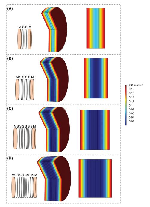
Fig. 3 COMSOL modeling of the stack scaffolds. COMSOL modeling of stacks of (A) two scaffolds, (B) four scaffolds, (C) six scaffolds, and (D) eight scaffolds utilizing parameters from the final scaffold holder design. "M" denotes medium and "S" denotes silk scaffold.
