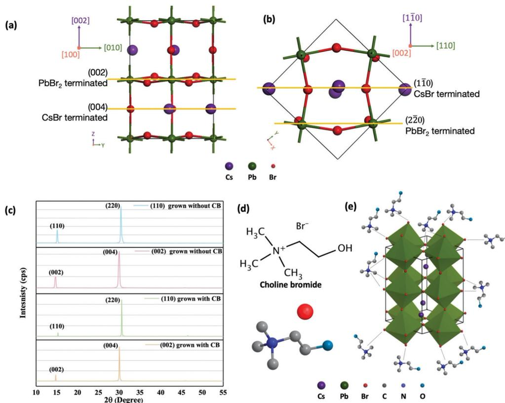
Fig. 2 (a) Side view of the orthorhombic CsPbBr<sub>3</sub> unit cell structure. The yellow lines indicate (002) and (004) plane. (b) Top view of the unit cell structure. The yellow lines indicate (110) and (220) plane. (c) XRD pattern of CsPbBr<sub>3</sub> single crystal grown with and without CB. (d) Molecular structure of choline bromide (CB). (e) Schematic illustration of CB assisted CsPbBr<sub>3</sub> single crystal growth.
