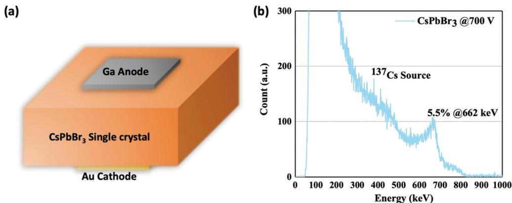
Fig. 4 (a) Schematic of detector structure (4.5 mm  $\times$  4.5 mm electrode area, 2.5 mm thickness). (b) 662 keV  $^{137}\text{Cs}$  spectrum acquired by CsPbBr<sub>3</sub> single crystal under 700 V.
