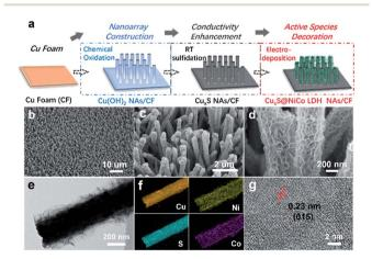
Fig. 1 (a) Schematic illustration of the preparation of  $Cu_xS@NiCo-LDHs$  core—shell composites. (LDH for layered double hydroxide, NA for nanoarrays, and RT for room temperature). (b–d) SEM images, (e) TEM image, (f) Elemental mappings of  $Cu_xS@Ni_{0.75}Co_{0.25}O_mH_n$ . (g) HRTEM image of ultra-thin  $Ni_{0.75}Co_{0.25}-LDH$ .
