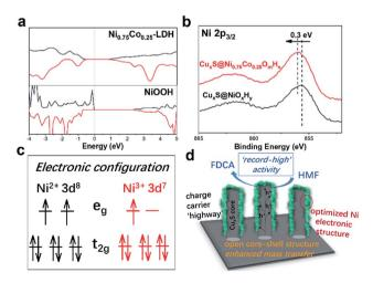
Fig. 4 (a) Projected density of states calculations for Ni<sub>0.75</sub>Co<sub>0.25</sub>-LDH and NiOOH. (b) High resolution Ni 2p<sub>3/2</sub> XPS spectra of Cu<sub>x</sub>S@Ni<sub>0.75</sub>- $Co_{0.25}O_mH_n$  and  $Cu_xS@NiO_mH_n$ . (c) Schematic illustration of the electronic configuration of the Ni cations with valence states of +2 and +3. (d) Schematic illustration of factors contributing to the high HMF oxidation activity.
