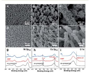
Fig. 6 SEM images of  $Cu_xS@Ni_{0.75}Co_{0.25}O_mH_n$  after catalyzing long-term HMF oxidation (a–c) and HER (d–f). Ni  $2p_{3/2}$  (g), Co  $2p_{3/2}$  (h) and O 1s (i) XPS spectra of  $Cu_xS@Ni_{0.75}Co_{0.25}O_mH_n$  after catalyzing long-term HMF oxidation (labeled as 'HMF') and hydrogen evolution reaction (labeled as 'H<sub>2</sub>').
