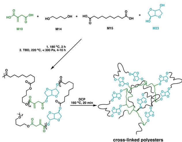
Fig. 18 Shape-memory cross-linked copolyesters synthesised using **M10**, **M14**, **M15** and **M23**.<sup>128</sup>
