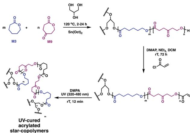
Fig. 14 Synthesis of biodegradable photo-cross-linked elastomers based on **M9** and **M3**.<sup>81</sup>
