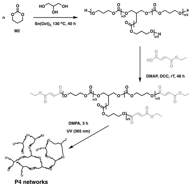
Fig. 13 Synthesis of **P4** networks through UV cross-linking of fumaric acid monoethyl ester-functionalised **P4** oligomers.<sup>77</sup>
