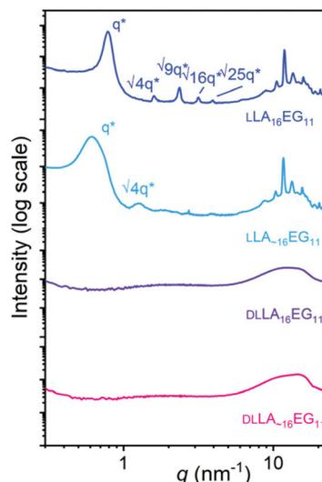
Fig. 2 Wide-angle X-ray scattering (WAXS) data for  $\text{LLA}_{16}\text{EG}_{11}$  (blue),  $\text{LLA}_{\sim 16}\text{EG}_{11}$  (light blue),  $\text{DLA}_{16}\text{EG}_{11}$  (purple),  $\text{DLA}_{\sim 16}\text{EG}_{11}$  (pink). The data is shifted vertically for clarity. Higher order Bragg reflections are indicated if present.
