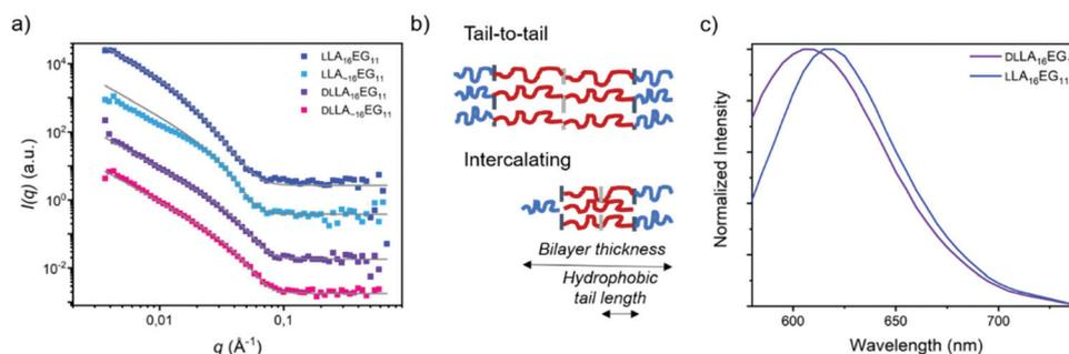
**Fig. 5** (a) SANS scattering profiles and corresponding fits in  $D_2O$ ,  $1 \text{ mg mL}^{-1}$ . Data is shifted vertically for clarity. (b) Schematic representation of possible bilayer structures in solution,  $LA_{16}$  in red,  $EG_{11}$  in blue. (c) Normalized emission spectra of the dye NR in self-assembled  $DLLA_{16}EG_{11}$  and  $LLA_{16}EG_{11}$  in water.
