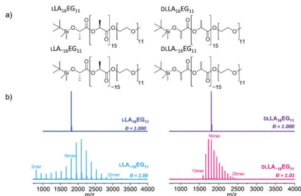
Fig. 1 (a) Chemical structures of studied BCOs: crystalline discrete  $LA_{16}EG_{11}$ , crystalline disperse  $LA_{\sim 16}EG_{11}$ , amorphous discrete  $DLLA_{16}EG_{11}$  and amorphous disperse  $DLLA_{\sim 16}EG_{11}$ . (b) MALDI-ToF spectra of all BCOs.
