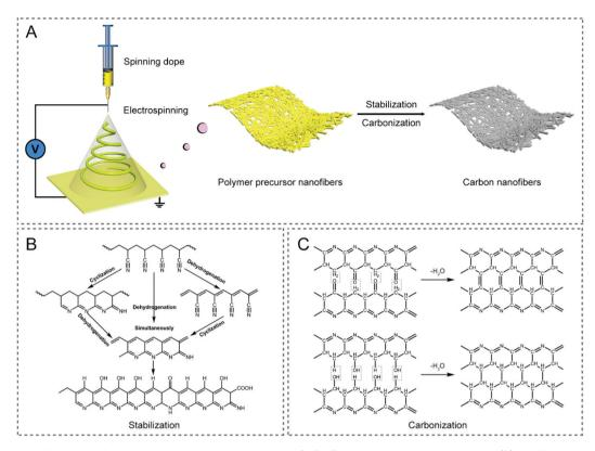
Fig. 1 (A) Schematic illustration of the preparation route of electrospun CNFs. Typical chemical reactions in the (B) stabilization and (C) carbonization processes of the PAN precursor.<sup>13,17</sup>
