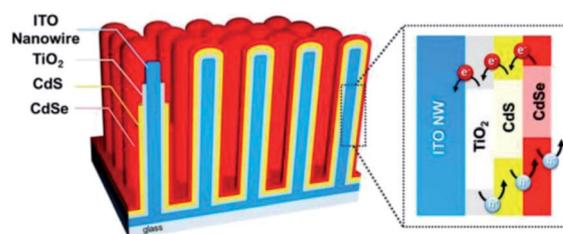
Fig. 6 Schematic illustration of the CdSe/CdS/TiO<sub>2</sub>/ITO multi-shell photoanode. Reproduced with permission from ref. 77; Copyright (2016) American Chemical Society.
