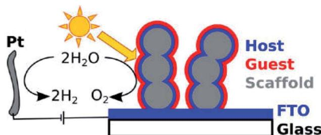
Fig. 4 Illustration of the host-guest PEC system by coating hematite films on Nb:SnO<sub>2</sub>. Reproduced with permission from ref. 71; Copyright (2012) American Chemical Society.
