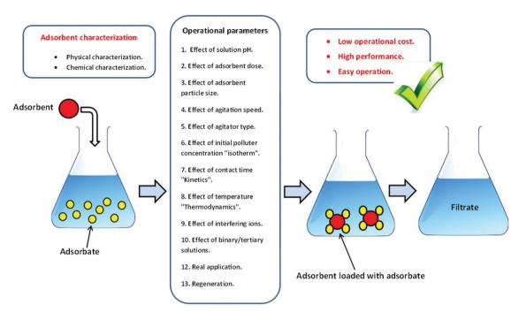
Fig. 4 Schematic diagram of batch adsorption.
