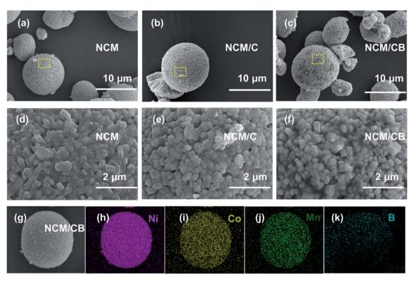
Fig. 2 The SEM images of NCM (a and d), NCM/C (b and e) and NCM/CB (c and f), the SEM image and corresponding elemental mapping of NCM/CB (q-k).
