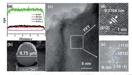
Fig. 3 The Element distribution obtained by EDS line scan (a), cross-sectional image (b), HRTEM images (c), enlarged version of HRTEM image (d) and FFT (e) for NCM/CB.
