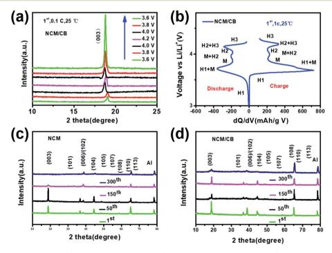
Fig. 8 (a) Ex situ XRD patterns of NCM/CB during the first charging/discharging procedure at 0.1C. (b) Corresponding charging/discharging curves. The ex situ XRD patterns of NCM/CB (c) and NCM (d) electrodes at dissimilar cycles at 1.0C.
