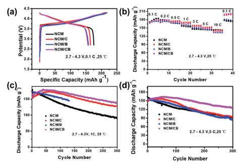
Fig. 5 Primary charge/discharge profiles (a), rate performance profiles (b), cycle performance at 1.0C (c) and 5.0C (d) for the samples.
