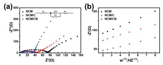
Fig. 7 (a) EIS spectra before cycling. (b) Connection between real parts of the complex impedance and  $\omega^{-1/2}$ .
