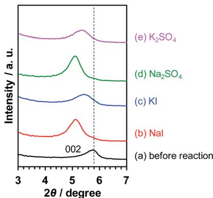
Fig. 5 002 diffraction peaks of Pt/KCa<sub>2</sub>Nb<sub>3</sub>O<sub>10</sub> in XRD (a) before reaction and after reaction in aqueous (b) NaI (10 mM), (c) KI (10 mM), (d) Na<sub>2</sub>SO<sub>4</sub> (5 mM), and (e) K<sub>2</sub>SO<sub>4</sub> (5 mM) solution.
