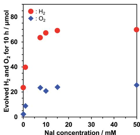
Fig. 4 Dependence of the photocatalytic water splitting activity of  $Pt/KCa_2Nb_3O_{10}$  on the NaI concentration. Reaction conditions: catalyst, 50 mg; reaction solution, 100 mL; light source, a 300 W Xe lamp ( $\lambda \geq 300$  nm).
