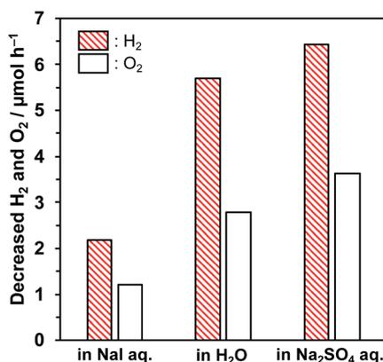
Fig. 3 Decreasing rates of  $H_2$  and  $O_2$  evolution over  $Pt/KCa_2Nb_3O_{10}$  in aqueous NaI solution (10 mM), pure water, and  $Na_2SO_4$  solution (5 mM) under dark conditions. Reaction conditions: photocatalyst, 50 mg; reactant volume, 100 mL; introduced amount of  $H_2$ , ca. 200  $\mu\text{mol}$  and  $O_2$ , ca. 100  $\mu\text{mol}$ .
