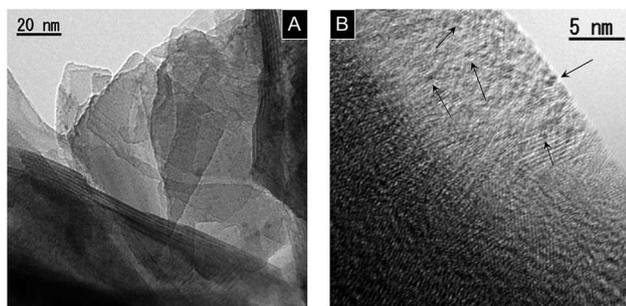
Fig. 1 TEM images of 1.0 wt% Pt/KCa<sub>2</sub>Nb<sub>3</sub>O<sub>10</sub> restacked nanosheets. (A) Lower and (B) higher magnification images. Arrows in (B) indicate some deposited Pt nanoclusters.
