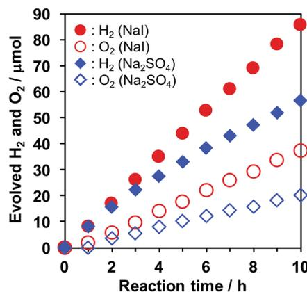
Fig. 2 Time courses of H<sub>2</sub> and O<sub>2</sub> evolution over Pt/KCa<sub>2</sub>Nb<sub>3</sub>O<sub>10</sub> in aqueous solution containing NaI (10 mM, red marks) or Na<sub>2</sub>SO<sub>4</sub> (5 mM, blue marks). Closed marks: H<sub>2</sub>; open marks: O<sub>2</sub>. Reaction conditions: catalyst, 50 mg; reaction solution, 100 mL; light source, a 300 W Xe lamp ( $\lambda \geq 300$  nm).
