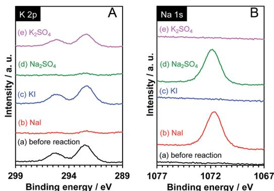
Fig. 6 XPS spectra for (A) K 2p and (B) Na 1s of Pt/KCa<sub>2</sub>Nb<sub>3</sub>O<sub>10</sub> (a) before and after reaction in aqueous (b) NaI (10 mM), (c) KI (10 mM), (d) Na<sub>2</sub>SO<sub>4</sub> (5 mM), and (e) K<sub>2</sub>SO<sub>4</sub> (5 mM) solution.
