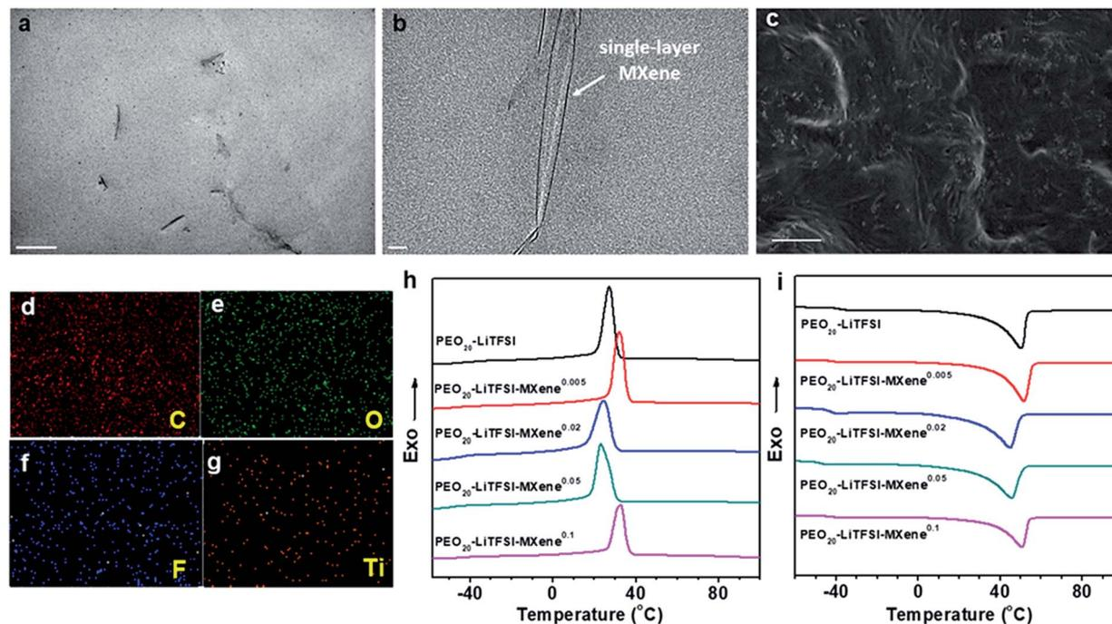
Fig. 2 TEM micrographs of the cross-section of PEO<sub>20</sub>-LiTFSI-MXene<sup>0.02</sup> ((a), scale bar is 500 nm; (b), scale bar is 20 nm). SEM image ((c), scale bar is 3  $\mu\text{m}$ ) and SEM-EDS surface scan of C (d), O (e), F (f) and Ti elements (g) in the cross-section of PEO<sub>20</sub>-LiTFSI-MXene<sup>0.05</sup>. DSC thermograms obtained at a rate of 10  $^{\circ}\text{C min}^{-1}$  during first cooling (h) and second heating (i).
