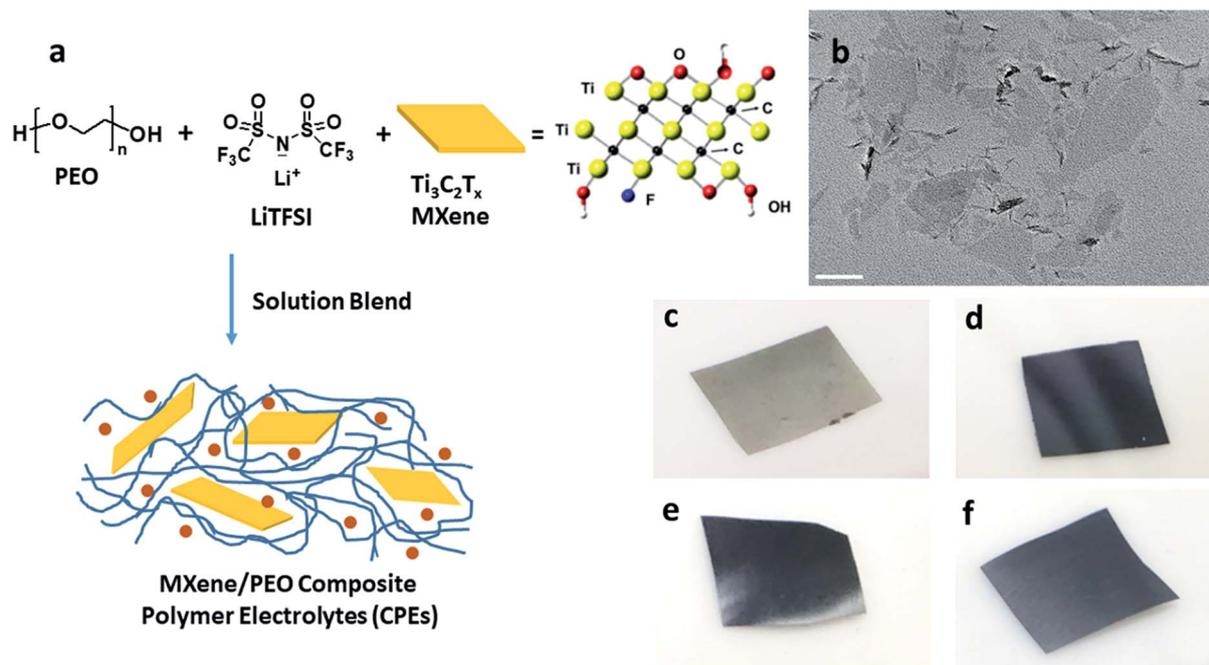
Fig. 1 Fabrication of MCPEs. (a) Preparation procedure of MCPEs. (b) TEM micrograph of the as-prepared few-layer MXene, scale bar is 100 nm. (c–f) Photographs of the MCPE membranes, (c)  $\text{PEO}_{20}\text{-LiTFSI-MXene}^{0.005}$ , (d)  $\text{PEO}_{20}\text{-LiTFSI-MXene}^{0.02}$ , (e)  $\text{PEO}_{20}\text{-LiTFSI-MXene}^{0.05}$  and (f)  $\text{PEO}_{20}\text{-LiTFSI-MXene}^{0.1}$ .
