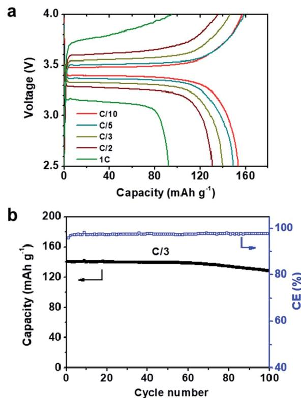
Fig. 4 Performance of the LiFePO<sub>4</sub>|PEO<sub>20</sub>-LiTFSI-MXene<sup>0.02</sup>|Li battery at 60 °C. (a) Voltage profile at different C rates. (b) Capacity and coulombic efficiency vs. cycle number at C/3. The LiFePO<sub>4</sub> loading is  $\approx 2.88$  mg cm<sup>-2</sup>.
