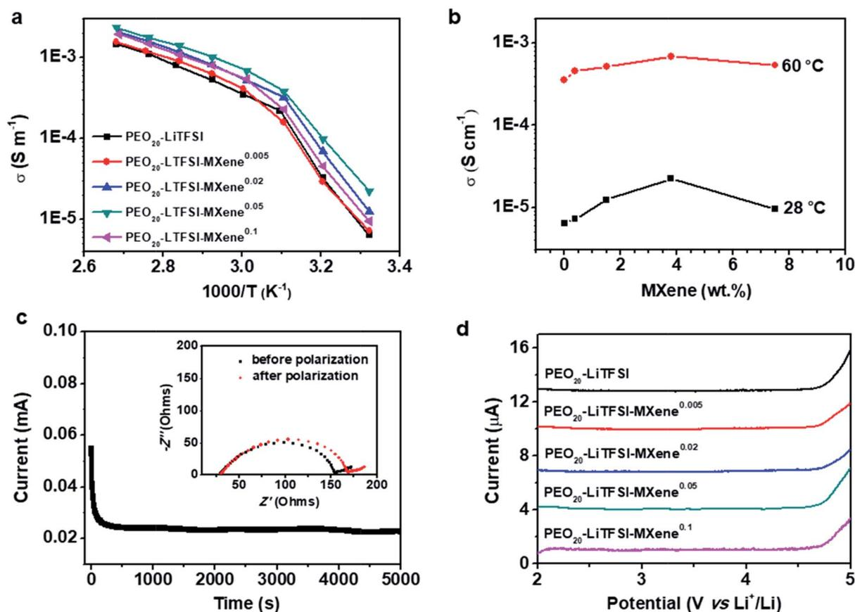
Fig. 3 (a) Temperature scan of the ionic conductivities of the MCPES. (b) Ionic conductivities vs. MXene content at  $28^\circ\text{C}$  and  $60^\circ\text{C}$ . (c) Lithium transference number measurement of the PEO<sub>20</sub>-LiTFSI-MXene<sup>0.02</sup>. (d) Linear sweep voltammetry of the MCPES (scan rate  $0.1\text{ mV s}^{-1}$ ). Curves are shifted along the current axis for clarity.
