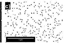
Fig. 7 (a) SEM secondary electron image of an area within a grain having some precipitates. (b) The same SEM image as in (a), with improved contrast upon applying the FFT filter. (c) The same SEM image as in (b), after performing background subtraction. The number density and area coverage of precipitates were calculated on the images after background subtraction.
