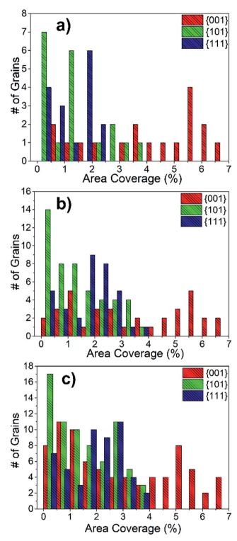
Fig. 9 The total distribution of precipitate area coverage on differently oriented grains at the surface of LSC64 pellets annealed at 800 °C for 2 h and 5 h. The grain orientations were processed with (a) 10°, (b) 15° and (c) 17.5° tolerance angles from the three major orientations.
