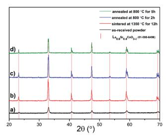
Fig. 1 XRD patterns of LSC64: (a) the as-received powder, (b) the pellet sintered in air at  $1350\,^{\circ}$ C for  $12\,h$ , and the pellet annealed in air at  $800\,^{\circ}$ C for (c) 2 h and (d) 5 h. The stick pattern of cubic R3m LSC64, PDF 01-080-6496, is also added.
