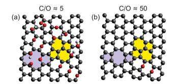
Fig. 1 Schematic representation of functionalized graphene at different degrees of reduction as indicated. Besides the functionalization of the basal plane of graphene through epoxy and hydroxyl groups as well as ketones, also a divacancy (light violet) and a Stone-Wales defect (yellow) are shown as representative examples of lattice defects. The red dots indicate oxygen and light grey ones hydrogen atoms
