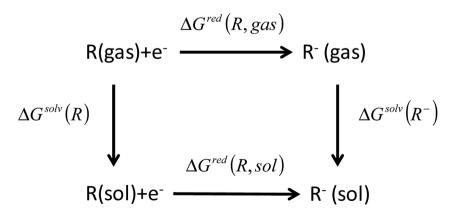
Fig. 2 Thermodynamic cycle used to calculate the equilibrium redox potential in the condensed phase.<sup>33,34</sup>
