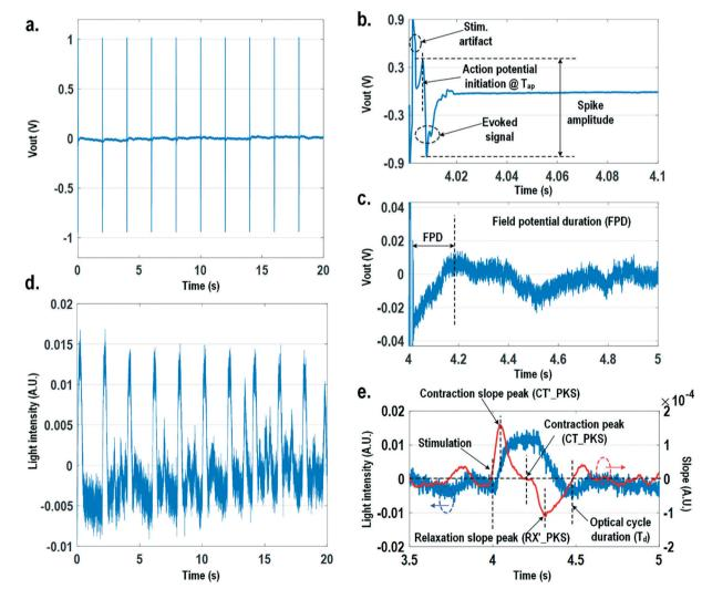
Fig. 8 (a) The measured extracellular potentials with concurrent stimulation at 0.5 Hz. (b) The zoomed-in view of the measured extracellular action potential spike. (c) The zoomed-in view of the measured extracellular T-wave. (d) The measured optical signals with concurrent stimulation at 0.5 Hz. (e) The zoomed-in view of the measured optical signal with its time derivative.
