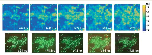
Fig. 5 Measured time-lapse impedance images of on-chip cultured rat cardiomyocyte spheroids together with reference fluorescence images. The cellular impedance measurement is performed at 100 kHz and the impedance magnitude is plotted.
