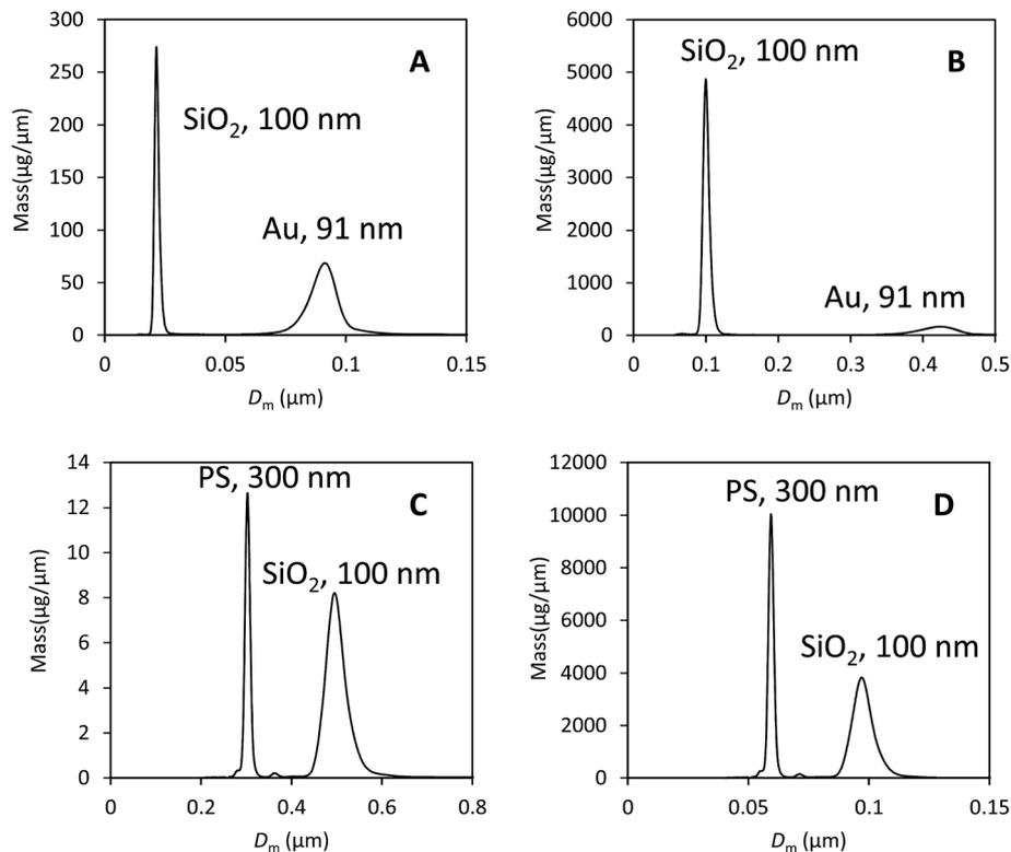
**Fig. 3** Binary mixtures of particles analysed by DCS. (A) Gold and silica particles of approximately equal diameter analysed using parameters for gold. (B) Data as panel (A) but analysed using parameters for silica. (C) Polystyrene (PS) and silica particles analysed using parameters for PS. (D) Data as panel (C) but analysed using parameters for silica.
