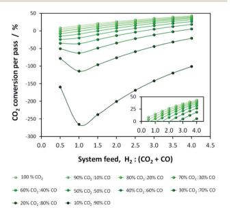
Fig. 3 Equilibrium  $\text{CO}_2$  conversion in the direct DME process (no recycle) at 250  $^{\circ}\text{C}$  and 50 bar.
