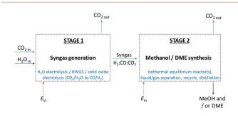
Fig. 1 Principal stages in methanol and DME syntheses from  $CO_2$  and  $H_2O$ . In Stage 1,  $CO_2$  and  $H_2O$  are converted to CO and  $CO_2$  and  $CO_3$  it utilised directly only  $CO_3$  is generated in Stage 1. In Stage 2, syngas is converted to methanol and/or DME.
