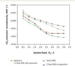
Fig. 12  $CO_2$  emissions normalised by the MEP for the methanol/DME production systems employing  $H_2$ –CO only (solid lines) and  $H_2$ – $CO_2$  only (dashed lines) feeds.
