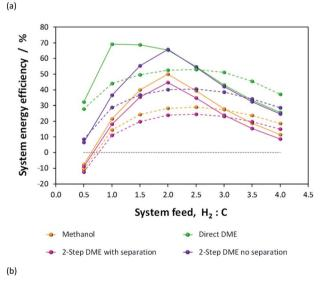
Fig. 9 Net energies obtained with (a) no energy savings and (b) maximum savings with the  $H_2$ -CO only (solid lines) and  $H_2$ -CO $_2$  only (dashed lines) system feeds for the four systems under investigation.
