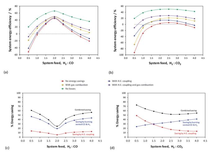
Fig. 8 Efficiencies for the methanol synthesis system for two extreme cases: (a) a  $H_2$ -CO only feed and (b) a  $H_2$ -CO<sub>2</sub> only feed. The 'no losses' scenario is a theoretical-only case in which the syngas conversion process consumes no energy and vented gases do not constitute energy loss. The corresponding energy savings made by coupling heat exchangers and by combustion of vented gases are shown in (c) and (d).
