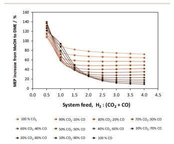
Fig. 6 MEP increase of the direct DME process relative to methanol alone; calculations based on reactor outputs at 250  $^{\circ}\text{C}$  and 50 bar in the absence of recycle.
