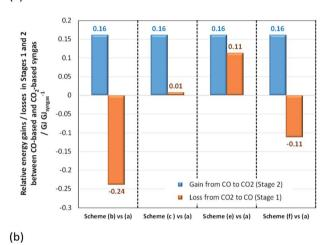
Fig. 14 Relative normalised energy losses in Stage 1 and gains in Stage 2 when (a) methanol and (b) direct DME systems are operated with CO-based and  $CO_2$ -based syngas.
