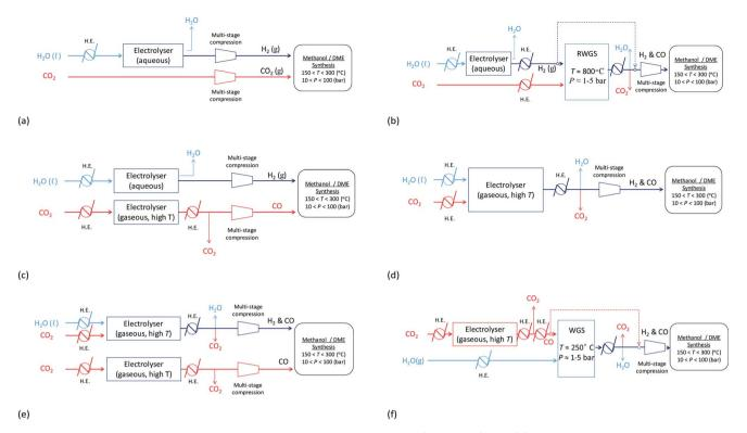
Possible routes for the production of syngas, with varying ratios of H<sub>2</sub>: C, from H<sub>2</sub>O and CO<sub>2</sub>.
