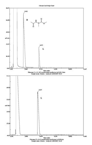
Fig. 1 Chiral GC data for Ac-DL-Ala-OMe and Ac-L-Ala-OMe (25 m  $\times$  0.25 mm, diethyl *tert*-butyldimethylisilyl- $\beta$ -cyclodextrin chiral capillary column).
