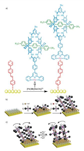
Fig. 21 (a) Schalley's rotaxane monolayer assembled using metallosupramolecular chemistry;<sup>57</sup> (b) a cartoon representation of the layer-by-layer deposition of Cl-responsive rotaxanes and (c) their proposed switching in the presence of Cl anions.<sup>58</sup> Adapted with permission from ref. 58. Copyright 2015 American Chemical Society
