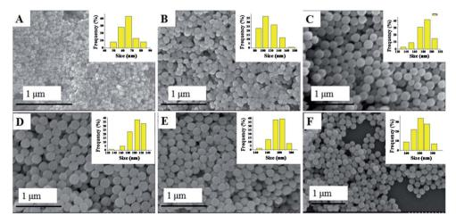
Fig. 2 SEM images of (A)  $Cu-CeO_2-Pt$ ; (B)  $Cu_{0.66}Co_{0.34}-CeO_2-Pt$ ; (C)  $Cu_{0.50}Co_{0.50}-CeO_2-Pt$ ; (D)  $Cu_{0.34}Co_{0.66}-CeO_2-Pt$ ; (E)  $Co-CeO_2-Pt$ ; (F)  $CeO_2-Pt$ .
