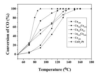
Fig. 8 CO conversion curves of Cu<sub>x</sub>Co<sub>1-x</sub>-CeO<sub>2</sub>-Pt and CeO<sub>2</sub>-Pt.
