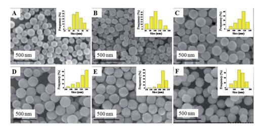
Fig. 1 SEM images of (A) Cu-CeO<sub>2</sub>; (B) Cu<sub>0.66</sub>Co<sub>0.34</sub>-CeO<sub>2</sub>; (C) Cu<sub>0.50</sub>Co<sub>0.50</sub>-CeO<sub>2</sub>; (D) Cu<sub>0.34</sub>Co<sub>0.66</sub>-CeO<sub>2</sub>; (E) Co-CeO<sub>2</sub>; (F) CeO<sub>2</sub>.
