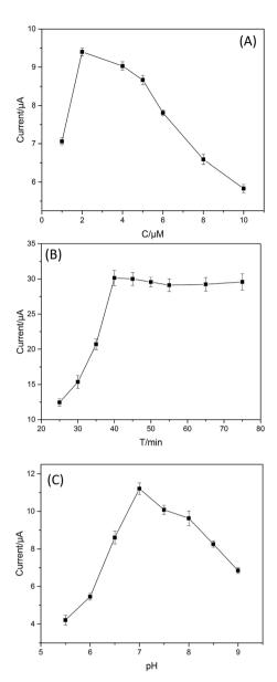
Fig. 4 (A) The optimum concentration of the aptamer; (B) the optimum incubation time; (C) the optimum pH of PBS.
