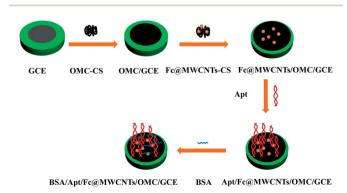
Scheme 1 Stepwise preparation of the aptasensor.
