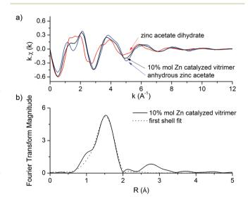
Fig. 4 (a) EXAFS spectra of zinc acetate dihydrate (red), anhydrous zinc acetate (blue) and the 10 mol% Zn-catalyzed epoxy-acid vitrimer system (black), (b) Radial structure functions of the 10 mol% Zn-catalyzed epoxy-acid vitrimer system (solid, black) and the first shell fit associated (dot, black).
