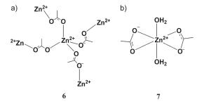
Fig. 3 Reference compounds used in EXAFS studies. (a) In compound 6: (ZnAc<sub>2</sub>) Zn<sup>2+</sup> is tetracoordinated with bridging acetate ligands. (b) In compound 7 (ZnAc2·2H2O) Zn2+ is hexacoordinated with bidentate acetate ligands and water.
