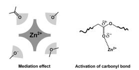
**Fig. 7** The two main actions of zinc as a catalyst in an epoxy-acid vitrimer network: mediation effect and ester activation designed from EXAFS and IR spectroscopy observations.
