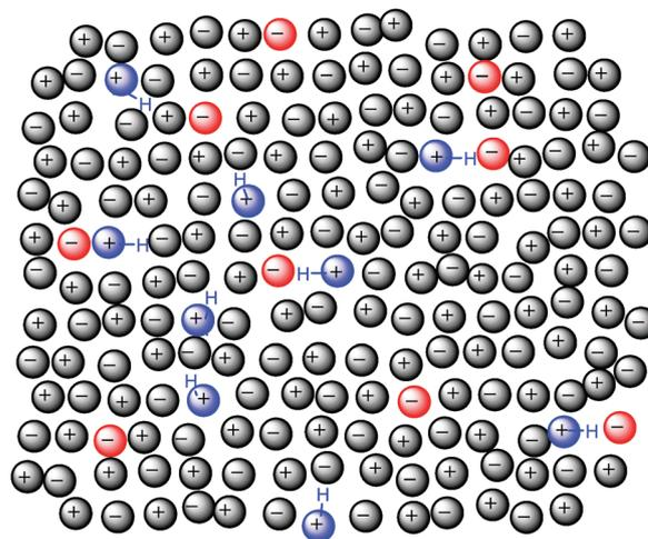
Fig. 8 Schematic ‘snapshot’ illustrating the preferential orientation of H-bonding within a randomly ordered ionic network for a reciprocal binary mixture  $[C_1]_x[C_2]_{1-x}[A_1]_x[A_2]_{1-x}$  where blue cations represent those with good H-bond donating groups and red anions are the strongest H-bond acceptors.
