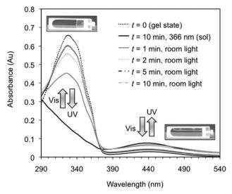
**Fig. 4** Reversible changes in the UV/Vis spectra for an organogel in toluene showing the reversible *trans*-to-*cis* isomerisation of the azobenzene moiety. On irradiation with UV light, the *trans* isomer changes to the *cis* isomer, leading to a gel-to-sol transition. Reproduced from ref. 47 with permission from the Royal Society of Chemistry.
