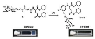
(a) Molecular structure of stilbene gemini surfactant gelator. Photographs of (a) the organogel (b) after irradiation (c) selective removal of part of the gel. Adapted from ref. 79 with the permission of the Royal Society of Chemistry,
