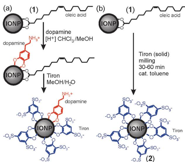
**Scheme 1** Synthesis of water-soluble IONPs by: (a) two-step ligand exchange in solution, leading to exchange of oleic acid ligands<sup>13</sup> and (b) herein demonstrated one-step mechanochemical solvent-free process.
