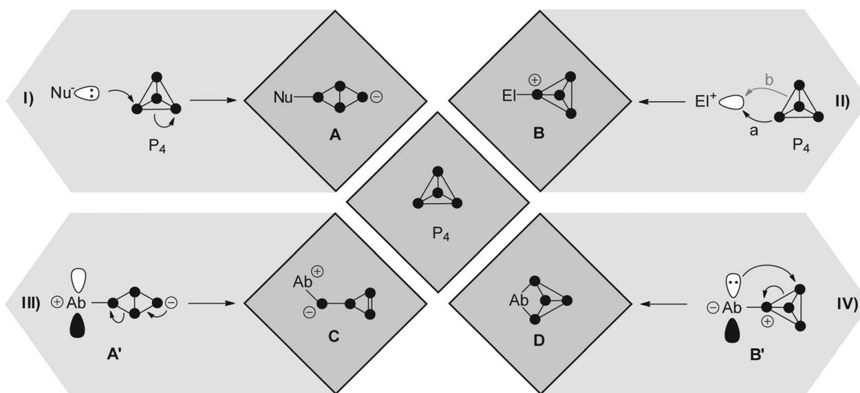
Fig. 1 Generalized reactions of  $P_4$  with nucleophiles (I,  $Nu^-$ ), electrophiles (II,  $El^+$ ), predominantly nucleophilic ambiphiles (III, Ab), and predominantly electrophilic ambiphiles (IV, Ab); **A–D** illustrate structural motifs obtained after reaction with the aforementioned species.
