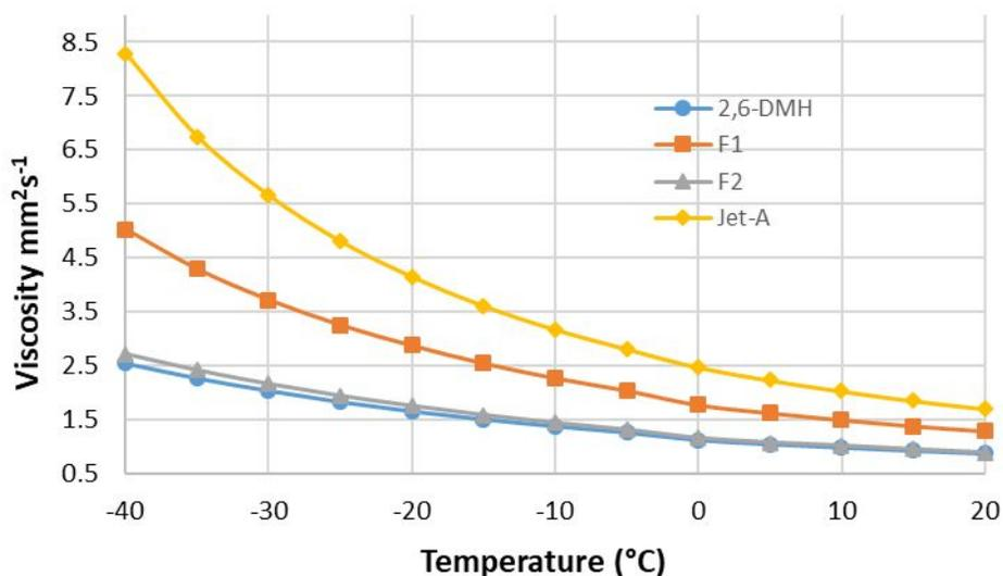
**Figure 2.** Kinematic viscosity of 2,6-DMH, F1, F2, and Jet-A from -40–20 °C
