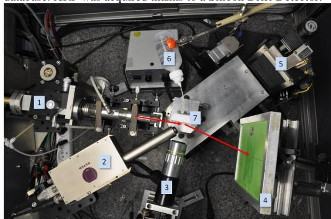
**Figure 2 :** *in situ* setup monitoring, rotating anode X-ray generator; 1. X-ray (Mo,  $\lambda_{\text{K}\alpha} = 0,709 \text{ \AA}$ ), 2. XRF detector, 3. OM, 4. Image plate, 5. Translation table, 6. Chlorinated solution, 7. Cell
