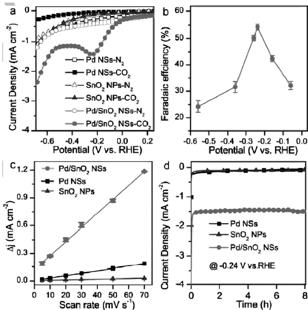
Fig. 14 Electrochemical characterization studies of Pd/SnO<sub>2</sub> NSs (Pd:Sn = 1:1) in comparison with Pd NSs and SnO<sub>2</sub> NPs. (a) LSV curves obtained in 0.1 M NaHCO<sub>3</sub> solution. (b) FE for CH<sub>3</sub>OH at various applied potentials. (c) Charging current density differences plotted against scan rates. (d) Chronoamperometry studies of different catalysts. Reprinted with permission from ref. 390. Copyright permission from 2018 Wiley-VCH Verlag GmbH & Co. KGaA, Weinheim.
