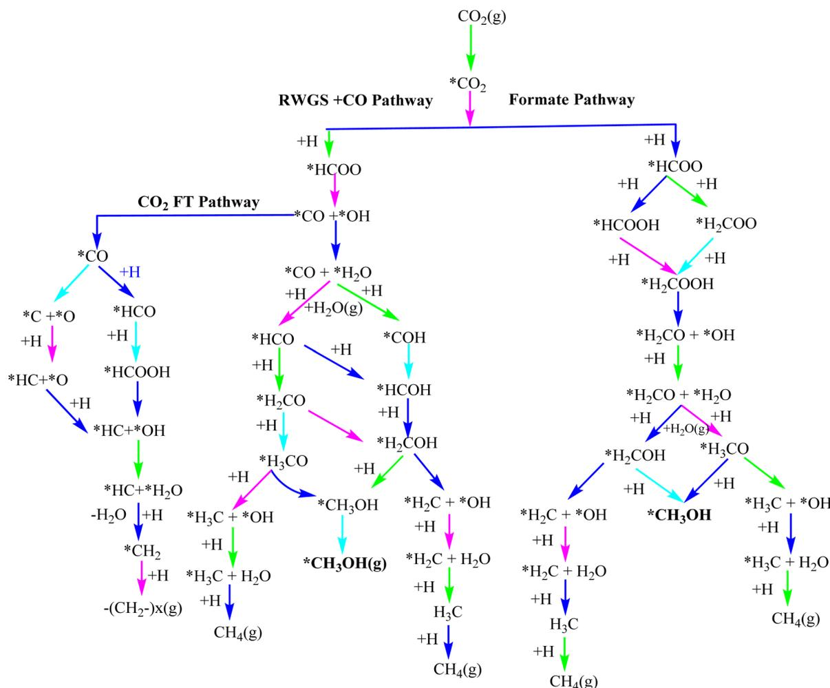
Fig. 6 Reaction mechanism of  $\text{CH}_3\text{OH}$  synthesis from  $\text{CO}_2$ .<sup>157</sup>
