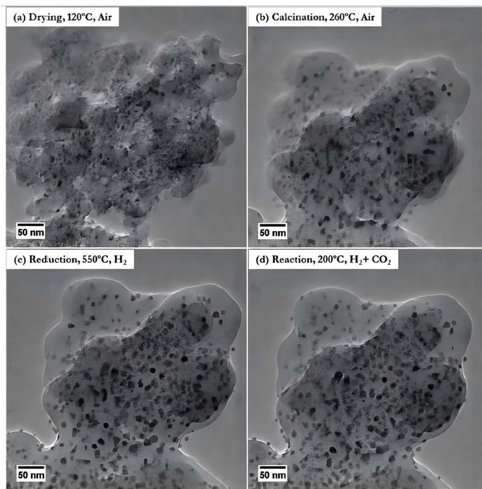
Fig. 13 IL-TEM images of the GaPd<sub>2</sub>/SiO<sub>2</sub> catalyst acquired after drying (a), calcination (b), reduction (c), and methanol synthesis (d).<sup>333</sup> Copyright 2015 American Chemical Society.
