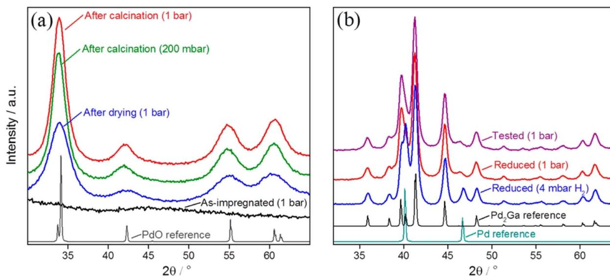
Fig. 12 (a) XRD patterns obtained from the impregnated, dried, and calcined catalyst precursor at room temperature and atmospheric pressure, and (b) from the reduced and tested GaPd<sub>2</sub>/SiO<sub>2</sub> catalyst for CO<sub>2</sub> hydrogenation. Reprinted with permission from ref. 333. Copyright 2015 American Chemical Society.
