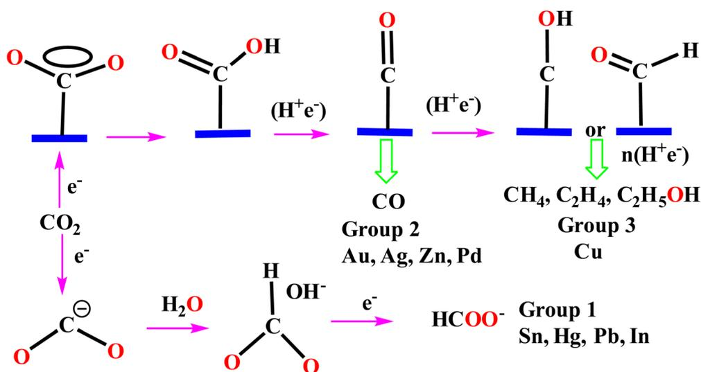
Fig. 5 Reaction mechanism of the electrochemical  $\text{CO}_2\text{RR}$  on metal electrodes in aqueous solutions.<sup>224</sup>
