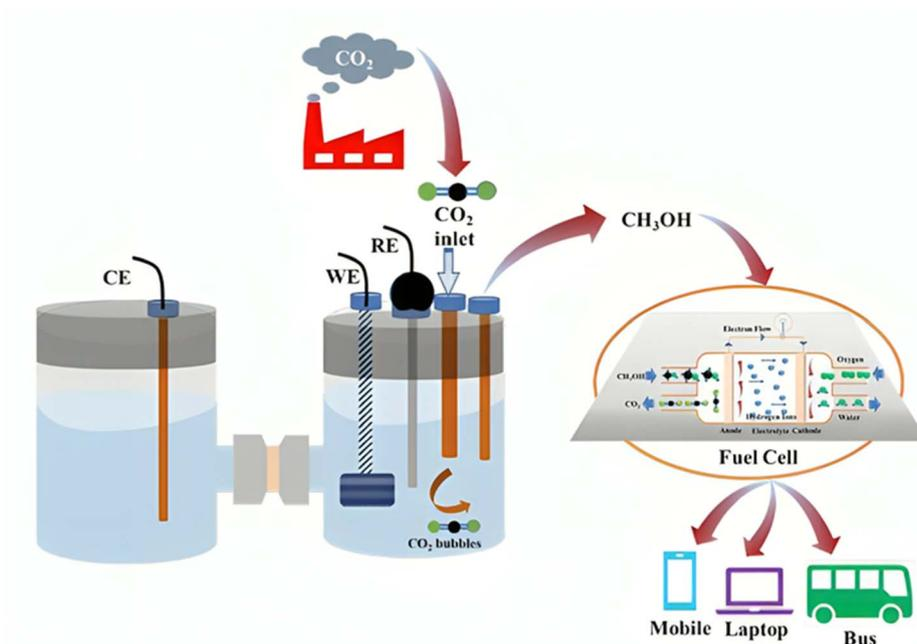
Fig. 4 Schematic representation of  $\text{ECO}_2\text{R}$  to  $\text{CH}_3\text{OH}$ .<sup>138</sup>
