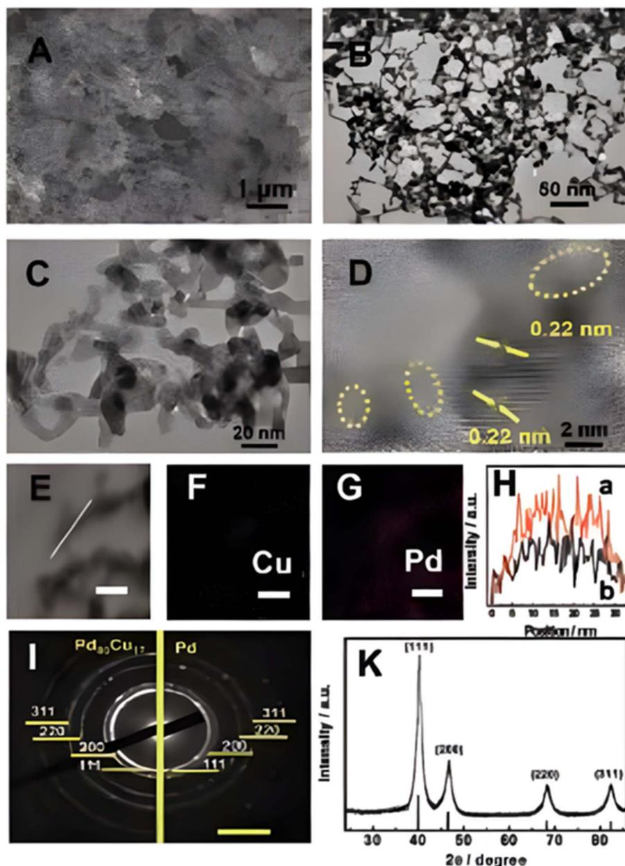
Fig. 15 (A) SEM, (B) and (C) TEM, (D) HR-TEM, and (E)–(G) EDX mapping images (scale bar: 20 nm). (H) Distribution of Pd (a) and Cu (b) in Pd<sub>83</sub>Cu<sub>17</sub> by line-scan analysis. (I) SAED pattern of the Pd<sub>83</sub>Cu<sub>17</sub> and pure Pd (scale bar: 10 1 nm<sup>−1</sup>). (K) XRD pattern of the Pd<sub>83</sub>Cu<sub>17</sub> aerogel. Reprinted with permission from ref. 389 Copyright permission from 2018 Wiley-VCH Verlag GmbH & Co. KGaA, Weinheim.
