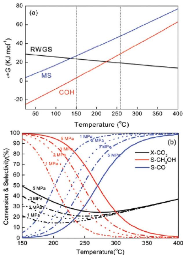
Fig. 3 (a) Free energy of methanol synthesis (MS) from CO<sub>2</sub>, RWGS and syngas hydrogenation (COH). (b) Equilibrium conversion-selectivity values of the CO<sub>2</sub>-hydrogenation reaction at various pressures. Reprinted with permission from ref. 156. Copyright 2020 Royal Society of Chemistry.
