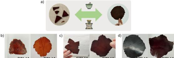
Fig. 7 Reprocessing scheme for the different materials. Resulting films for each formulation (b) EVS1, (c) EVS2 and (d) EVS3.
