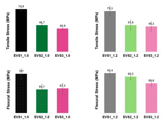
Fig. 8 Comparison of the mechanical properties of the six formulations studied herein. Tensile stress for (a) 1.0 formulation and (b) 1.2 formulation. Flexural stress for (c) 1.0 formulation and (d) 1.2 formulation.
