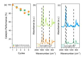
**Fig. 6** Catalytic performance within five cycles of *p*-NP reduction up on using 3Ag@Py-CH POP and 3Ag@TPA-CH POP (a) FTIR fresh and recovered 3Ag@Py-CH POP (b), FTIR of fresh and recovered 3Ag@TPA-CH POP (c).
