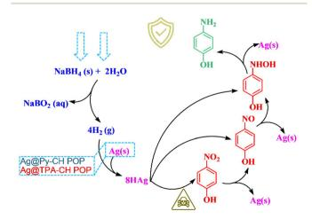
**Scheme 2** The proposed reduction mechanism of p-NP catalyzed Ag nanoparticles decorated CH-POPs nanocomposites.
