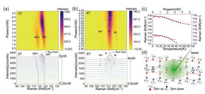
Fig. 2 (a) and (b) The laser power dependence Raman spectra of low-energy magnon-phonon (MP) branches in few-layer FePSe<sub>3</sub> at 0 T and 6 T, respectively. (c) The position of a Raman peak as a function of laser power and temperature at 0 T. Circles denote MP+ and squares denote MP-, with black indicating temperature-dependent parameters and red representing power-dependent parameters. (d) Schematic diagram of local tuning of magnon properties by laser heating.
