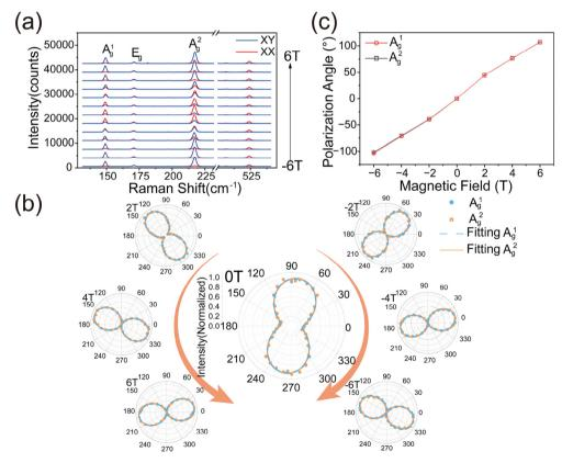
Fig. 4 (a) The parallel and perpendicular polarization Raman spectra of  $FePSe_3$  and Si with the magnetic field varying from -6 T to 6 T. (b) The linear polarization Raman spectrum of  $FePSe_3$  with the magnetic field varying from -6 T to 6 T. (c) The rotation angle of polar Raman.
