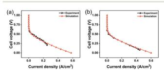
**Fig. 2** (a) Comparison of polarization curve with polarization curve obtained from simulation literature parameters<sup>54</sup> and (b) Comparison of polarization curve with polarization curve obtained from experimental literature parameters.<sup>55</sup>
