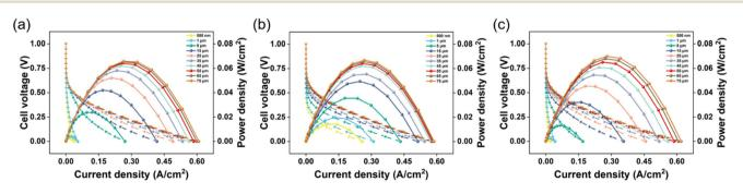
Fig. 4 Polarization curve obtained by changing the CL thickness: (a) change of anode CL thickness; (b) change of cathode CL thickness; (c) change of anode and cathode CLs thickness.
