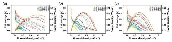
Fig. 3 Polarization curve obtained by changing the active specific surface area (Av): (a) anode CL; (b) cathode CL; (c) the anode and cathode CLs.
