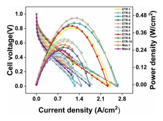
Fig. 8 Comparison between the top 10 El score data and the polarization curve of the original database.
