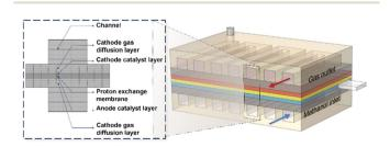
Fig. 1 3D geometric model of DMFC
