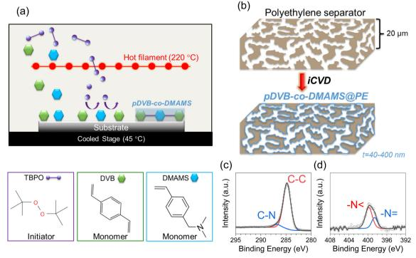
Fig. 1 (a) Schematic of iCVD-based synthesis of pDVB-co-DMAMS and chemical structures of initiator and monomers used. (b) Schematic of ideal iCVD deposition to form conformal polymer coatings on porous separators. Core-level (c) C 1s and (d) N 1s XPS spectra of iCVD-generated pDVBco-DMAMS deposited on planar Si substrates.
