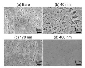
Fig. 2 Scanning electron micrographs of (a) bare polyethylene and (bd) 40 nm-, 170 nm-, and 400 nm-iCVD@PE separators, showing the topside relative to the orientation of the separator in the iCVD reactor.
