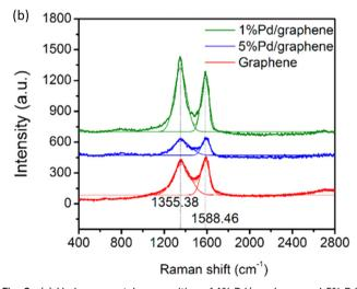
Fig. 8 (a) Hydrogen uptake capacities of 1% Pd/graphene and 5% Pd/ graphene functionalized graphene at various charging pressures. (b) Raman spectroscopy of graphene, 1% Pd/graphene, and 5% Pd/ graphene, showing D and G bands at ~1355.38 cm<sup>-1</sup> and ~1588.46 cm<sup>-1</sup>, respectively. This figure has been reproduced from ref. 106 with permission from American Chemical Society, copyright 2016.
