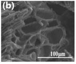
Fig. 13 (a and b) SEM images of activated carbon derived from corncob using various chemical activation methods. This figure has been reproduced from ref. 122 with permission from Elsevier, copyright 2010.
