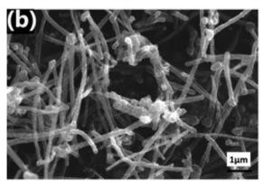
Fig. 12 SEM images of (a) pristine MWCNTs and (b) MWCNT:SnO<sub>2</sub> composites. This figure has been reproduced from ref. 174 with permission from Elsevier, copyright 2018.
