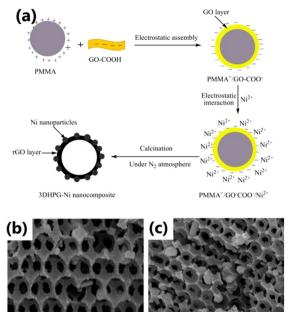
Fig. 9 (a) Schematic illustrating the synthesis for three-dimensional porous hierarchical graphene. (b and c) SEM images of three-dimensional porous hierarchical graphene. This figure has been reproduced from ref. 213 with permission from Elsevier, copyright 2018.
