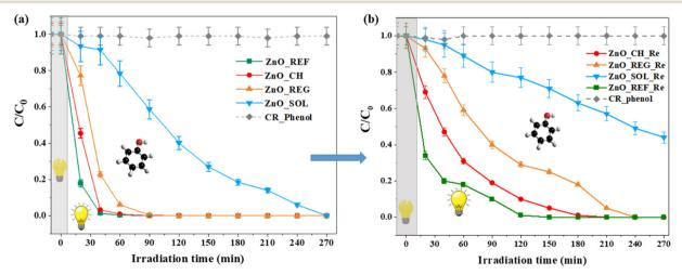
Fig. 7 Phenol degradation curves of ZnO NPs: a) before and after interaction with soil solutions (CR\_Phenol: phenol concentration without ZnO\_NPs); b) reusability test via phenol degradation.
