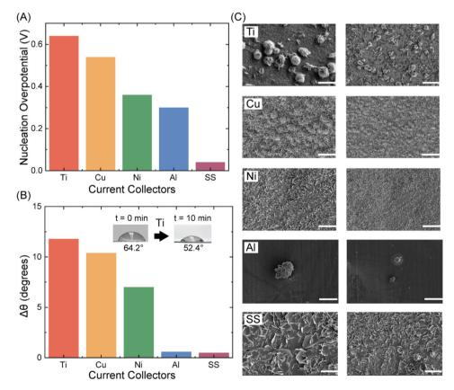
Fig. 3 (A) Nucleation overpotential for the galvanostatic plating of 0.5 mA h cm<sup>-2</sup> of Zn on Cu as a function of collector materials. (B) Variation in contact angle after 10 min on the different current collectors. (C) SEM images of 0.5 mA h cm<sup>-2</sup> deposited onto different current collectors. The scale bar for the panel on the left is 10 µm and for the panel on the right is 30 µm.
