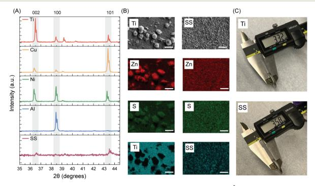
Fig. 4 (A) XRD spectra of electrodeposited Zn on different materials, at a fixed capacity of 0.5 mA h cm<sup>-2</sup>. (B) SEM and EDX mapping for Ti and SS. (Scale bar: 10  $\mu$ m.) (C) Thickness of Ti and SS coin cells is shown after 50 cycles.
