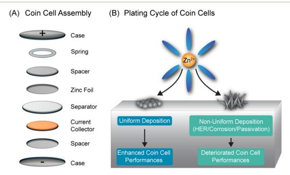
Fig. 1 (A) Schematic depicting different components of a coin cell. (B) Schematic illustrating the impact of Zn electrodeposition and side reactions on battery performance, influenced by various coin cell components.
