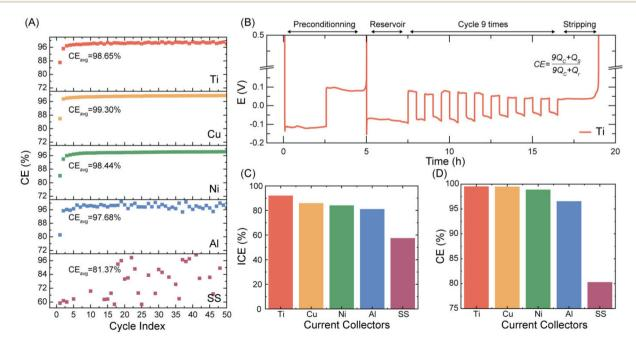
Fig. 2 (A) The Coulombic Efficiency (CE) of asymmetric cells with different current collector materials, over 50 cycles. (B) Representative potential vs. time (Aurbach) curve for Ti. (C) Initial Coulombic Efficiency (ICE) trends from the coin cell data. (D) Coulombic efficiency trends using Aurbach curve as shown in (B), as function of current collector materials.
