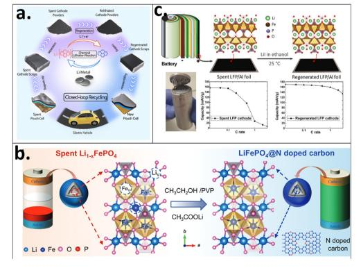
Fig. 5 Schematic representations of (a) direct chemical regeneration of LFP using polycyclic aryl-lithium compounds in ethylene glycol dimethyl ether,<sup>58</sup> (b) regeneration process using lithium acetate in ethanol,<sup>64</sup> and (c) direct LFP regeneration at room temperature in different organic solvents using lithium iodide.<sup>61</sup>
