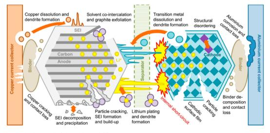
Fig. 2 Degradation mechanisms in LIBs (adapted from ref. 67).
