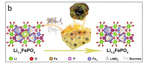
Fig. 6 (a) Solvent-free direct lithiation of spent LFP and other cathode materials at room temperature with very rapid reaction kinetics<sup>62</sup> and (b) direct LFP regeneration via a low-temperature molten salt process coupled with a reductive environment. 63
