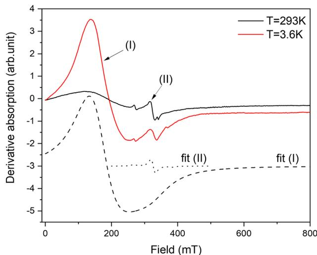
**Fig. 7** The experimental EPR spectra of powdered complex **2** recorded at  $T = 3.6$  K and 293 K (solid lines). The dashed lines represent fits of Co (II) in two different positions for a low temperature spectrum.
