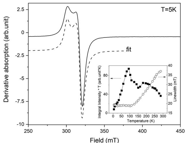
**Fig. 6** The experimental EPR spectrum of powdered complex **1** recorded at  $T = 5$  K (solid line). The dashed line represents the calculated absorption from the best fit. The inset shows the temperature evolution of integral intensity  $\times T$  (left vertical axis) and linewidth (right axis).
