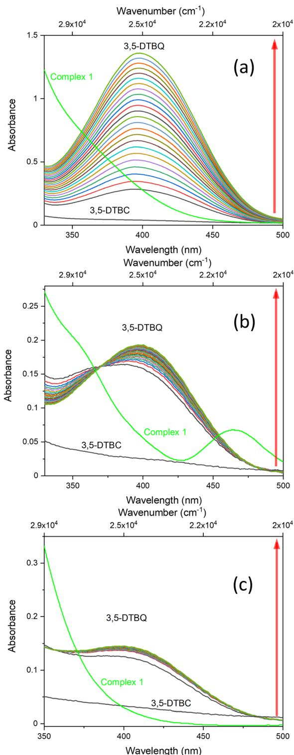
**Fig. 9** Spectral changes observed during the oxidation of 3,5-DTBC ( $1 \times 10^{-2}$  M) to the corresponding quinone in the presence of 1 ( $5 \times 10^{-5}$  M) in different solvents: (a) methanol, (b) acetonitrile and (c) dimethylsulfoxide.
