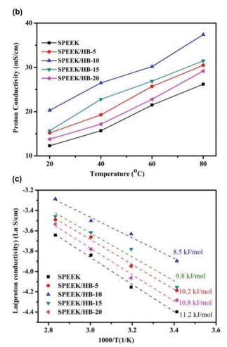
Fig. 11 (a) Illustration of HKUST-1 in sPEEK matrix, SP/CT-MOF-3, depicting hydrogen bond network, proton transport pathways and low methanol permeability. Reproduced with permission from ref. 100, Copyright 2018, Royal Society of Chemistry. (b) Proton conductivity and (c) Arrhenius plots of pristine SPEEK and HKUST-1/BPO4 in sPEEK matrix. Reproduced with permission from ref. 101, Copyright 2021, Wiley VCH.
