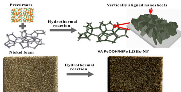
Fig. 9 Schematic illustration of the formation process of the porous VA FeOOH/NiFe LDH-NF electrodes. Reproduced with permission from ref. 86. Copyright 2016 American Chemical Society.
