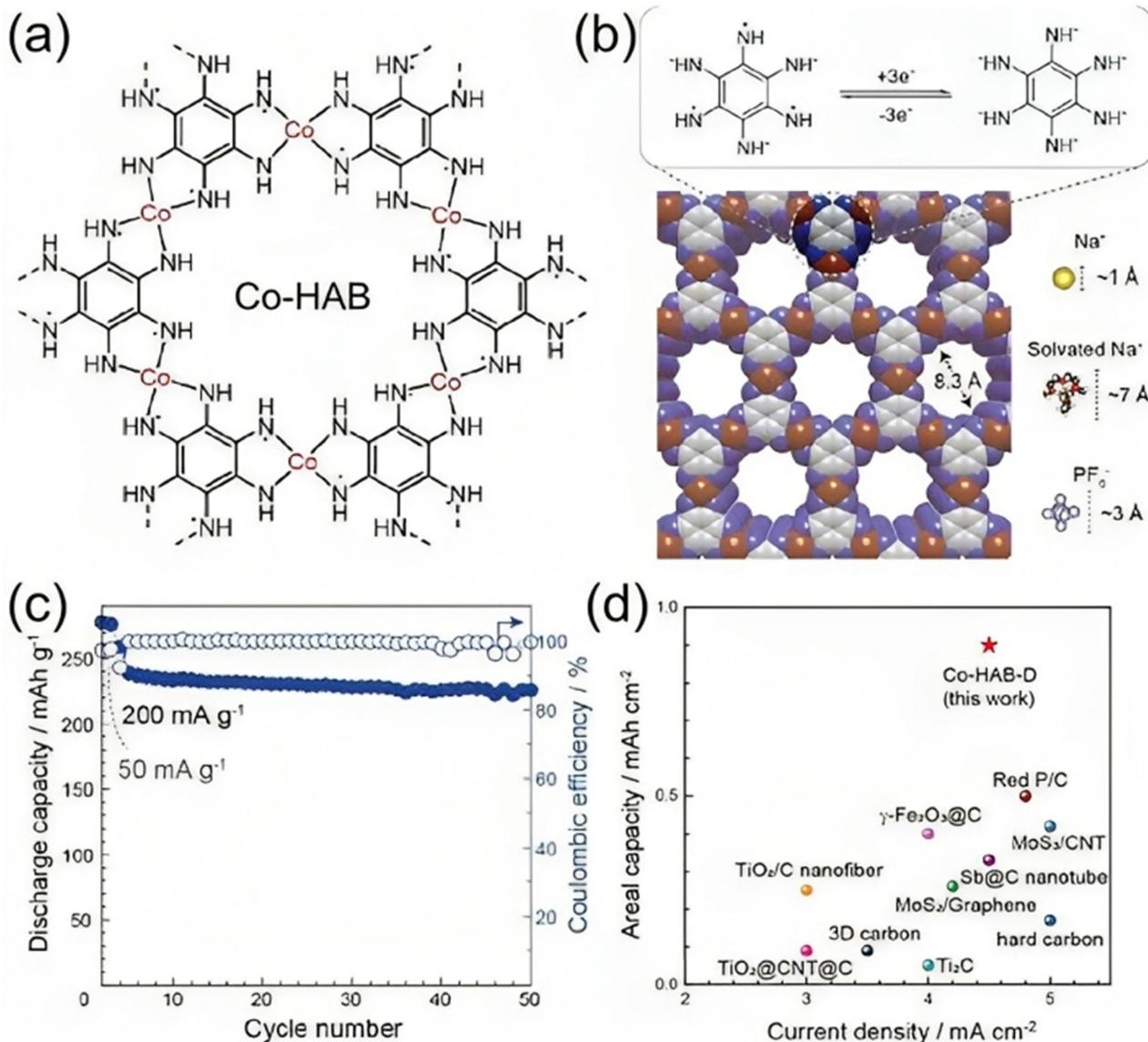
**Fig. 8** Electrochemical performance of the Co-HAB electrode for SIBs. (a) Chemical structure of Co-HAB. (b) A space-filling diagram of Co-HAB and the size comparison of the pore with  $\text{Na}^+$ , solvated  $\text{Na}^+$  and  $\text{PF}_6^-$  ions. Top: proposed three-electron reversible reaction of the HAB ligand in Co-HAB. (c) Cycling stability test of the Co-HAB electrode. (d) Comparison of areal capacity of Co-HAB with representative reported anode materials for SIBs.<sup>137</sup>
