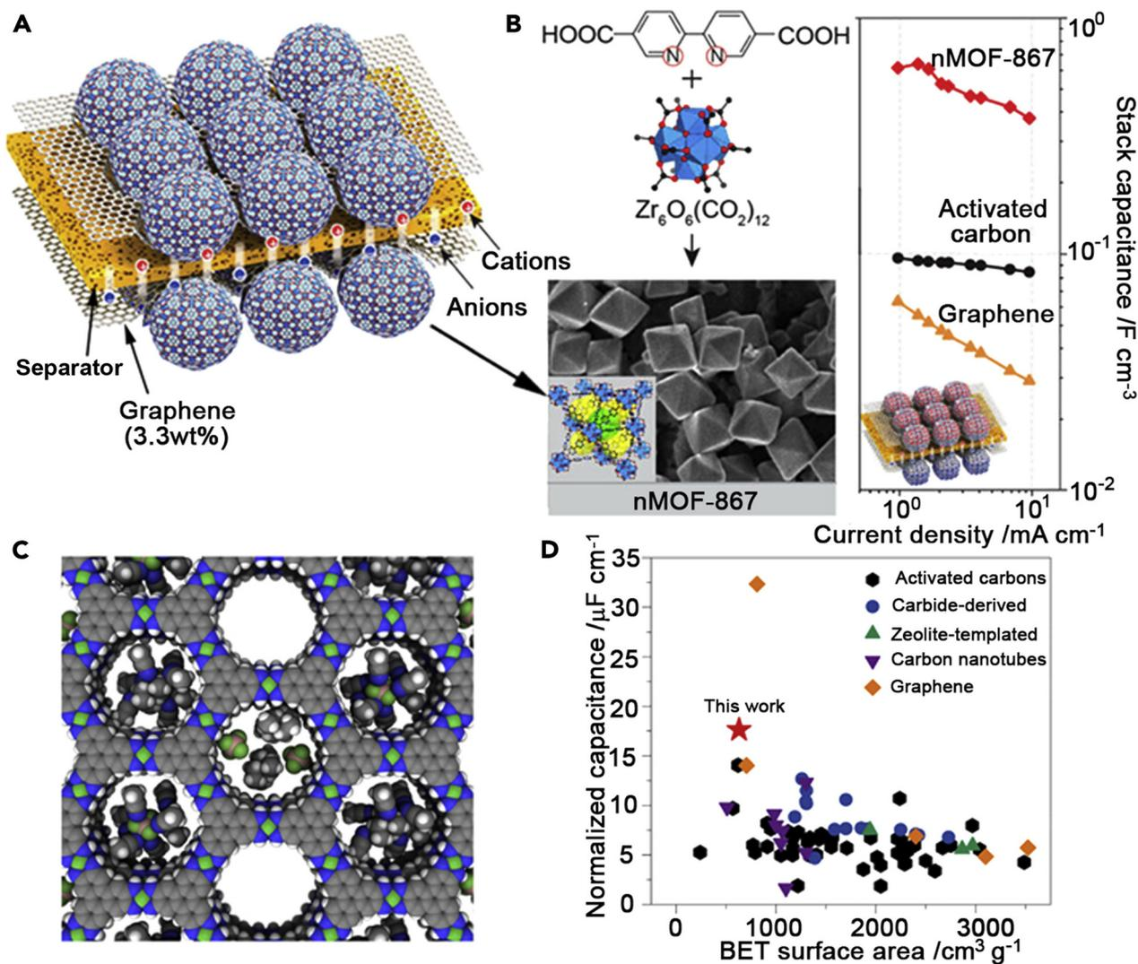
Fig. 3 MOF-based supercapacitors. (A) Schematic construction of MOF supercapacitors.<sup>53</sup> (B) Structure and nanocrystal morphology of nMOF-867 and comparison of stack capacitances among various EDLC materials.<sup>51</sup> (C) A space-filling diagram of idealized Ni<sub>3</sub>(HITP)<sub>2</sub> (Ni, green; F, lime; N, blue; C, gray; B, brown; H, white).<sup>51</sup> (D) Comparison of BET-surface-area-normalized areal capacitances among various EDLC materials.<sup>54</sup>
