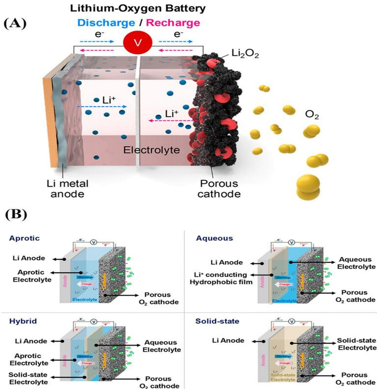
Fig. 9 (A) Schematic representation of a Li–O<sub>2</sub> battery. (B) Schematic configuration of all types of Li–O<sub>2</sub> cells.<sup>145</sup>
