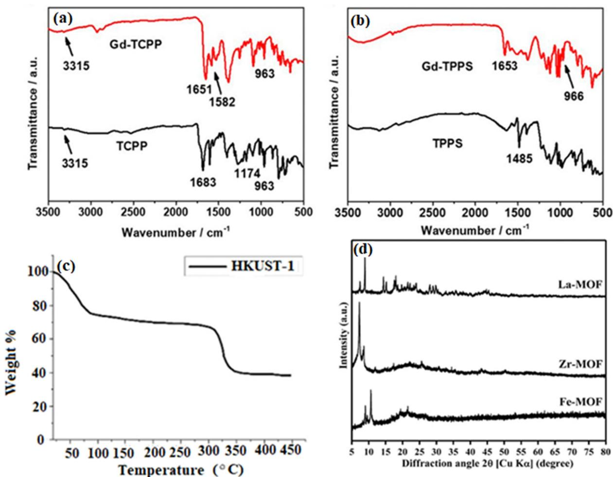
Fig. 2 (a) FT-IR analysis of TCPP and Gd-TCPP.<sup>34</sup> (b) FT-IR analysis of TPPS and Gd-TPPS. (c) Thermogravimetric analysis (TGA) of HKUST-1.<sup>35</sup> (d) Powder X-ray diffraction (PXRD) spectra of Fe-, Zr-, and La-based metal-organic frameworks derived from recycled PET plastic bottles.<sup>36</sup>
