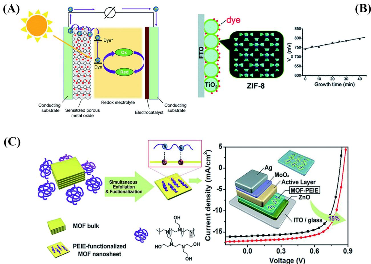
Fig. 4 (A) Schematic representation of typical dye-sensitized solar cells. (B) The use of MOFs for the photoanodes in DSSCs as the blocking layer.<sup>71</sup> (C) Schematic illustration of the preparation of 2D MOF nanosheets and their modified electron-extraction layer for photovoltaic devices.<sup>72</sup>
